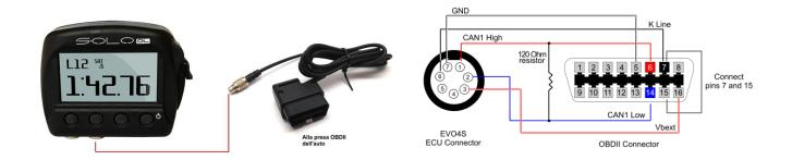
**Please note**: CAN termination resistor is integrated in the cable while K line pull-up resistor is integrated in SoloDL.
