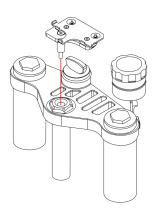
Screw the central screw on the hinge so that this last grips.
