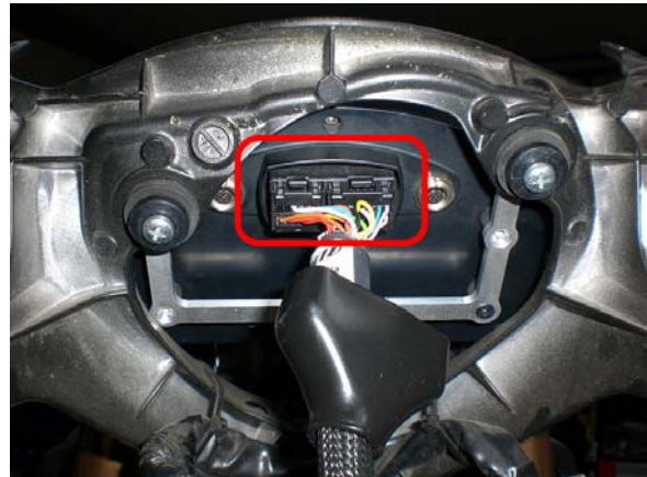
Figure 10 : MXL wiring connection.
