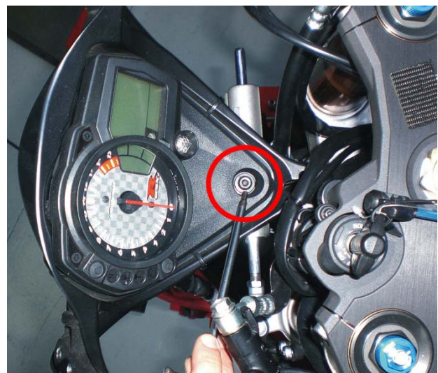
Figure 2: front fixing bolt of the stock dash.
