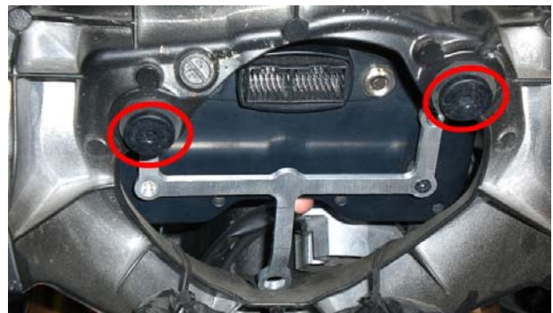
Figure 8: rear screws are fixed.
