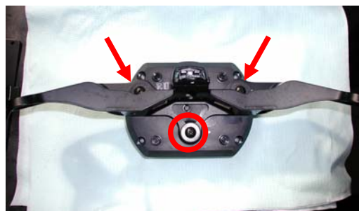
Figure 6: screws that fixes the stock dash
