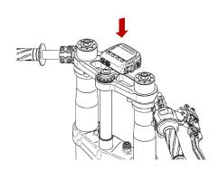
Tighten Solo bracket screws.
