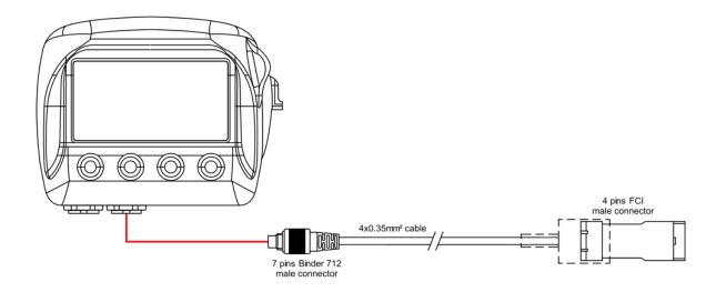
To connect AiM EVO4 to **V02563150** cable use the five pins Binder 712 female connector labelled "ECU" of the logger – third from the left on the top row –as shown here below.
