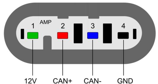
All AiM devices are provided with a 120 Ohm CAN termination resistor. To make them communicate with Nemesis TCS kit it is necessary to remove it. SoloDL and EVO4 resistor is on the ECU connection cable and it is thereby possible to remove it, while in all MXL the resistor is integrated and not removable. For this reason the wiring connection is different.
