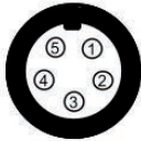
5 pins Binder 712 female connector pinout external view
