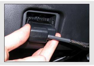
Now the system is powered and connected to the vehicle. It is only necessary to make MXL receive data from the ECU: connect the female plastic connector of the interface cable to:
