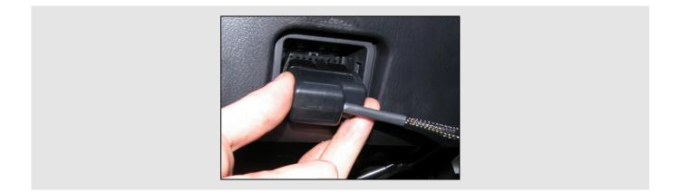
Now the system is powered and connected to the vehicle. It is only necessary to make MXL receive data from the ECU: connect the free cables of the interface cable as follows:
