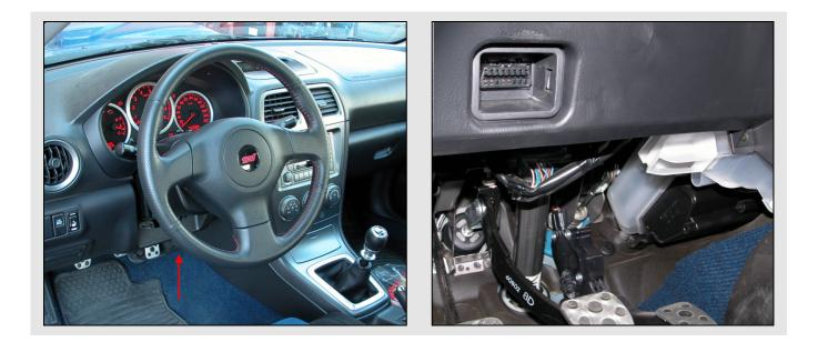
The image here below shows the Subaru interface wiring connector plugged in the OBDII plug.
