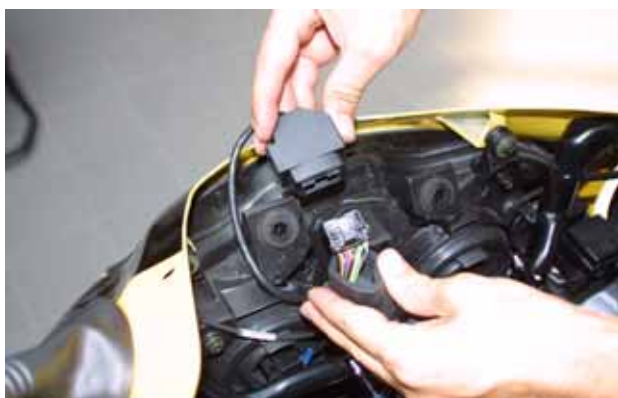
Figure 26: Wiring installation – particular of the AMP connector
