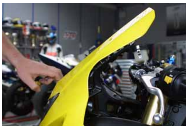
Figure 13: the fairing and the headlight screws have been slackened.
