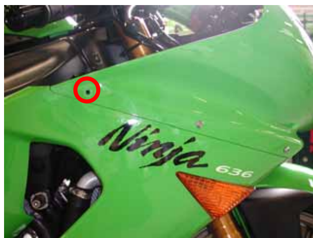
Figure 2: .Lateral screw to remove.
