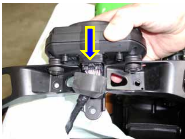
Figure 5: the on board wiring connector
