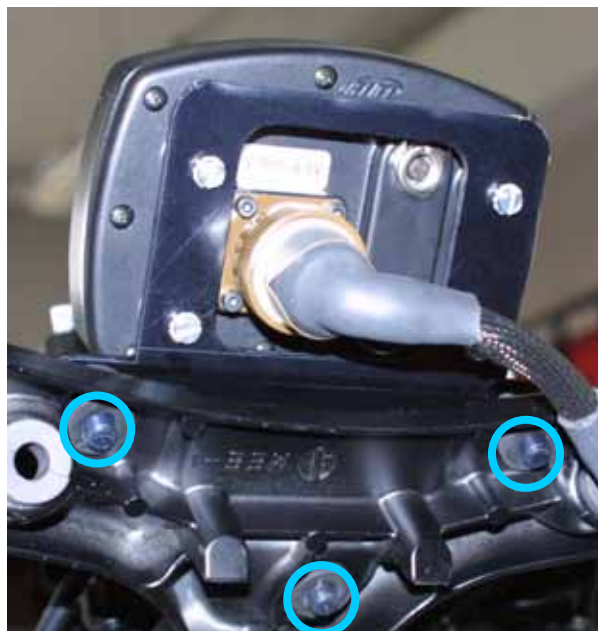
Figure 24: MyChron 3 Plus / Gold installed.
