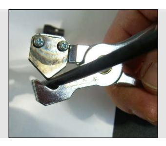
Insert the two locknuts in the cut part of the pipe as shown here below. If the plastic cover of the metal braid does not allow the locknut to slip peel the pipe.
