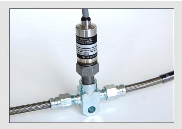
**Warning**: once the sensor installation has been completed ensure that the braking circuit is cleared and check its tightness.
