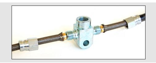
Tighten the threads a quarter turn at a time until the right position is reached; **be careful not to exceed 1,5 Kg (15 Nm)**.
